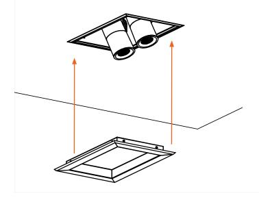
PUSH TRIM UP INTO THE HOUSING UNTIL SPRING LOADED FASTENERS HAVE RELEASED AND SECURED THE TRIM INTO PLACE
