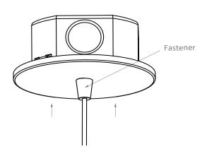
Align module with socket, push and rotate clockwise until module snaps in place and is secured.
