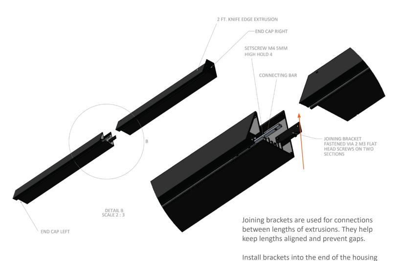
Install end caps where the end of the extrusion is exposed.
