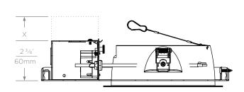
X ranges from 2  $^3/8$ " (60 mm) to 3  $^7/8$ " (99 mm) depending on emergency backup and high output models
