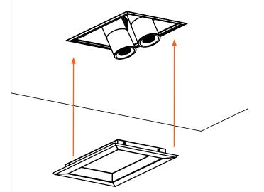
PUSH TRIM UP INTO THE HOUSING UNTIL SPRING LOADED FASTENERS HAVE RELEASED AND SECURED THE TRIM INTO PLACE
