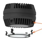
Place accessory in clip and proceed to snap 4 sides to module built in pockets in order to secure.
