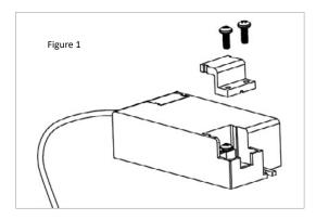
Remove round head M3 screws from the power supply driver to release the wiring plate (Figure 1).
