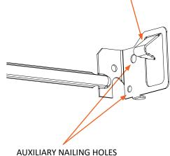
• MOUNT BRACKETS TO TRAY WITH PROVIDED FASTENERS.
