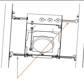
SECURE TRAY TO JOISTS OR C-CHANNEL USING THE MOUNTING BARS AS SHOWN. INSTALL MOUNTING BARS ONTO TRAY. PLACE TRAY IN DESIRED LOCATION.
