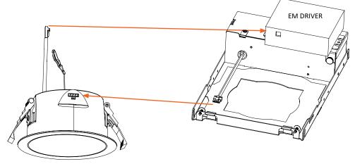
REMOTE EM INSTALLATION (FOR SEMI-DIFFUSED FLANGE AND BAFFLE - SD/SD ONLY)
