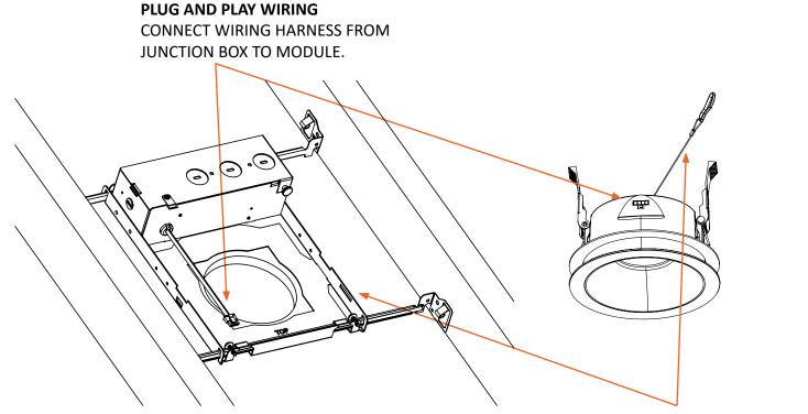
**IMPORTANT: SAFETY REQUIREMENT!** SECURE TETHER FROM MODULE TO TRAY.
